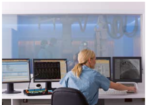
The control room glass switches from transparent to opaque, to maximize patient privacy
